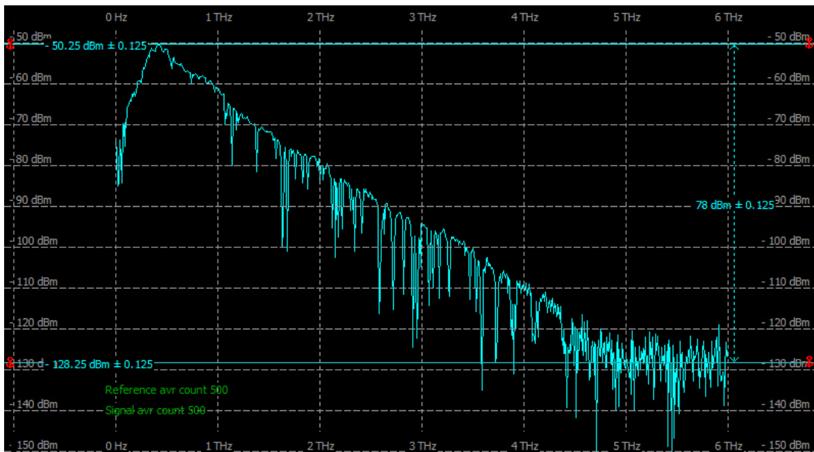
THz pulse FFT Spectrum in the air registered with the Terahertz Registration System TRS-16
