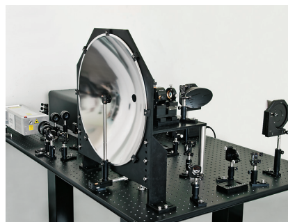
LIDAR operating in terahertz range was used to scan remote objects at 7 m distance. THz LIDAR installed in Lomonosov Moscow State University, Russia
